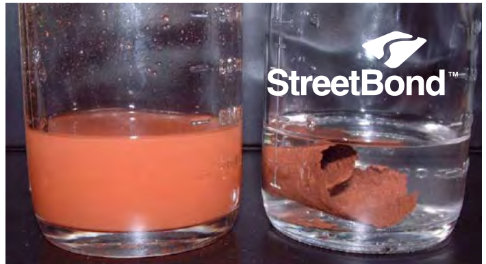
Fuel emulsion tests comparing regular polymer coating with StreetBond150. Streetbond is resistant to damage from fuel, oil, salts and de-icing agent exposure.
